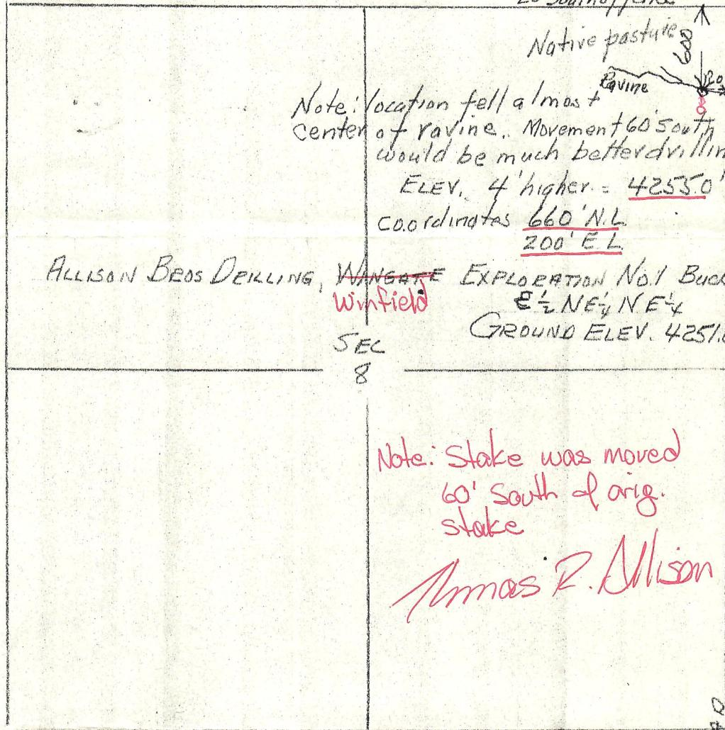
I hereby certify that the above plat is an accurate representation of a correct survey showing the location of Allison Bros. Drilling, Wingfield Exploration No.1 Buckleiter Oilwell in  $E\frac{1}{2}NE\frac{1}{4}NE\frac{1}{4}$  Sec. 8 T9N R54W 6PM. The elevation of the ground at the stake is 4251.0 feet above sea level from U.S.G.S. Bench Mark.
