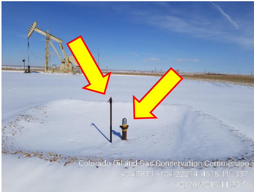
Photo 3 – Unmarked Risers
