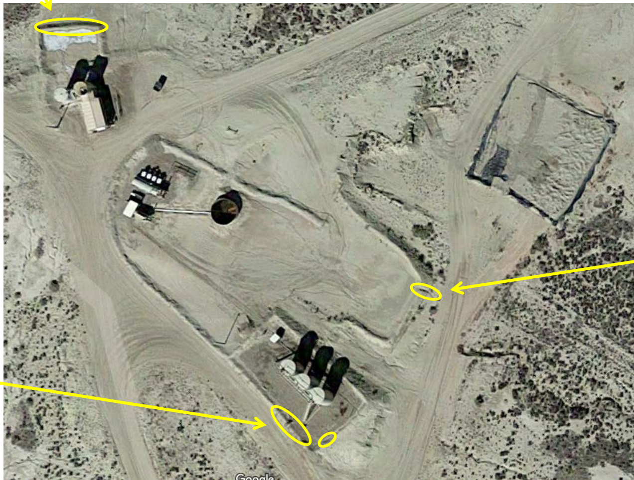
Photo 12. Tank battery – Inadequate berms circled in yellow.
