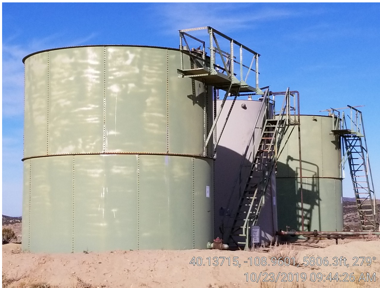
Photo 2. Central tank battery.
