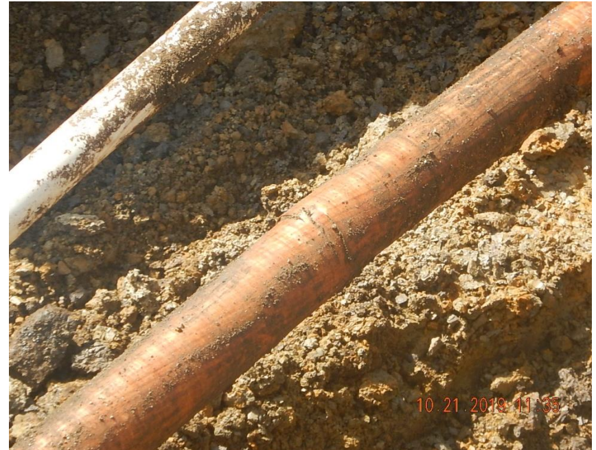
Close up view of failure identified on 3" fiberglass flowline (spiral type fracture).
