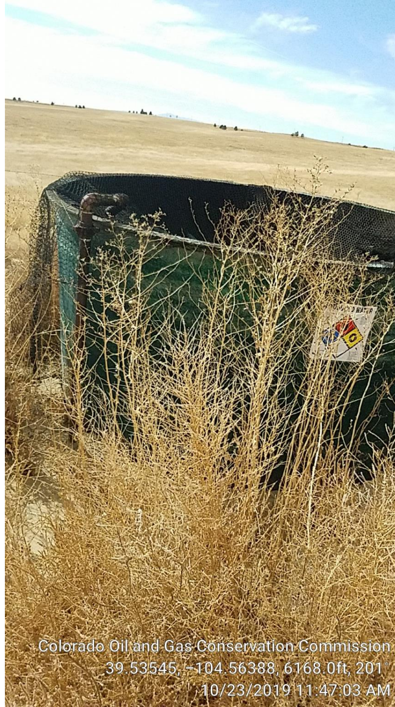
An 80 bbl, open topped, netted, fiberglass skim tank.
