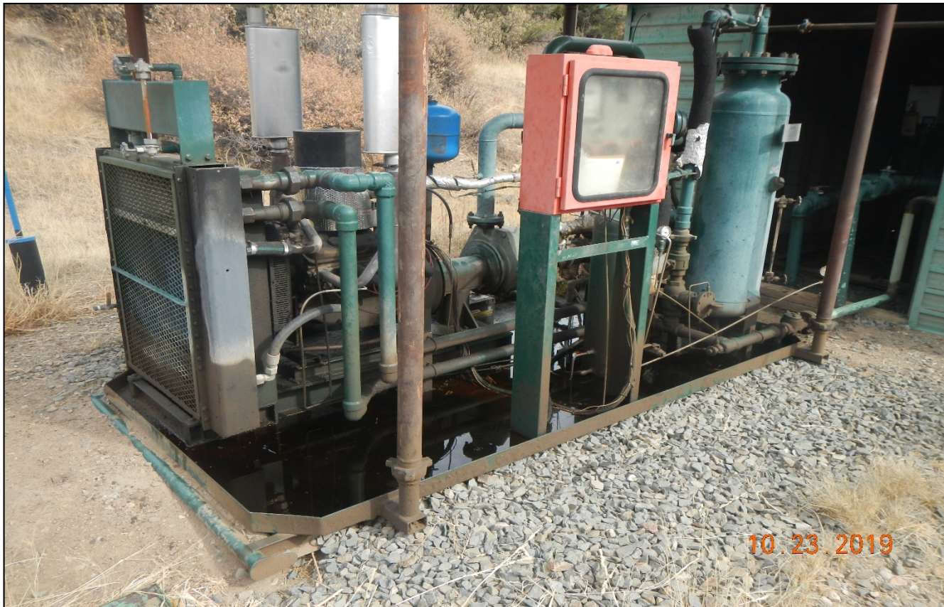
Photo 3. There is oil spilled into the engine skid.
