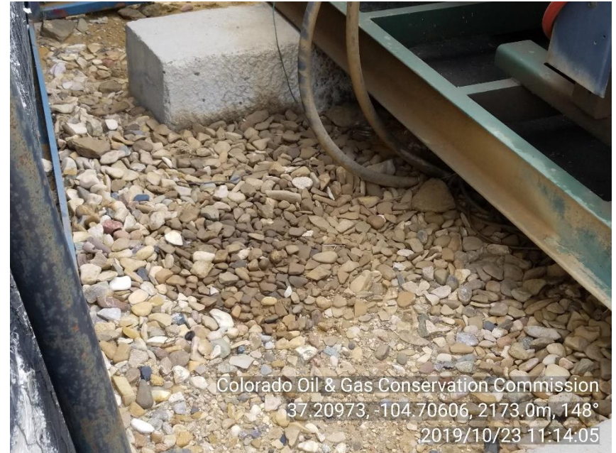
PHOTO 6: AREA OF IMPACTED SOIL NEAR ENGINE SKID. Properly treat or dispose of oily waste in accordance with 907.e. CA DATE 11-23-19.
