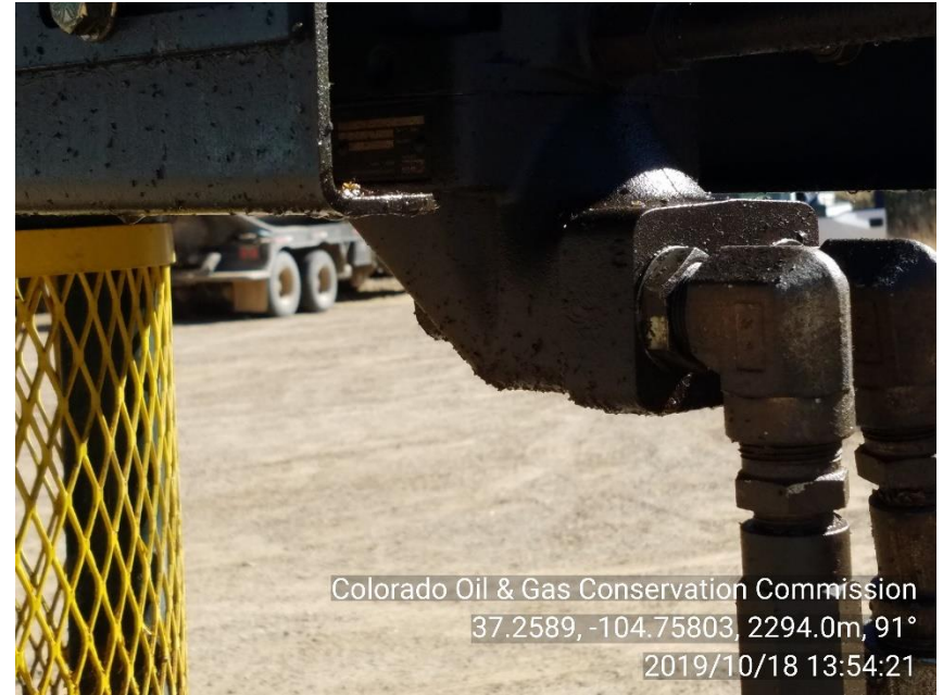
PHOTO 4: FITTING APPEAR TO ME LEAKING
