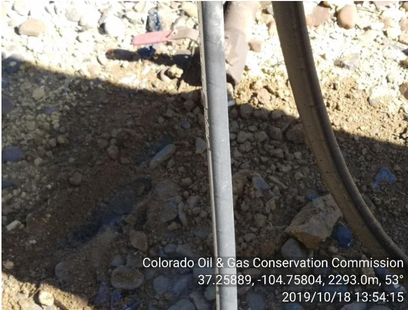
PHOTO 3: AREA OF IMPACTED SOIL NEAR ORIGINAL WELLHEAD APPEARS TO HAVE LEAKING HYDRAULIC HOSE OR QUICK FITTINGS. Properly treat or dispose of oily waste in accordance with 907.e. CA DATE 11-18-19
