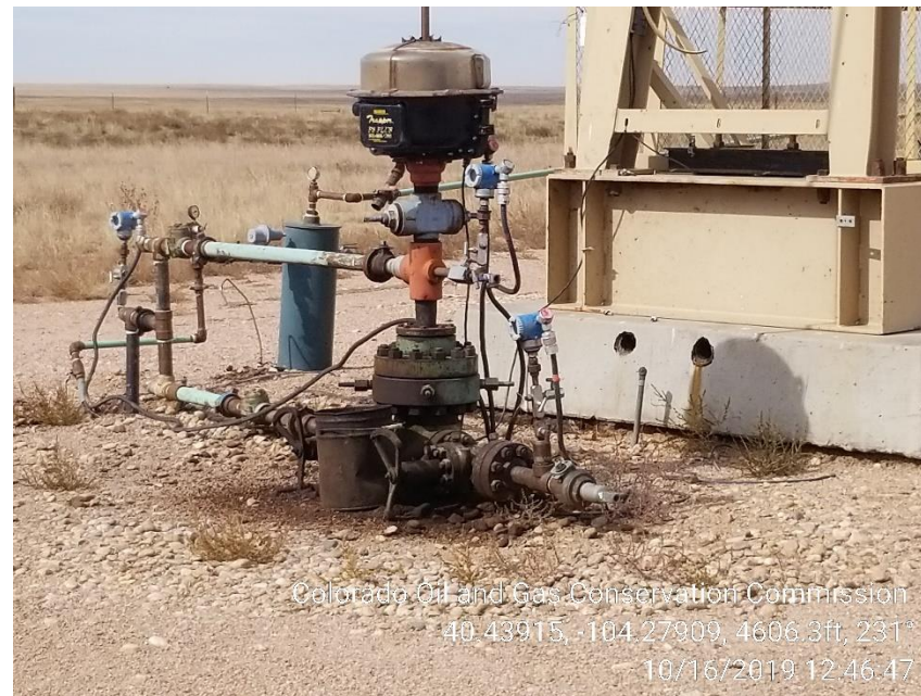
Photo 2 – Stained Soil at Wellhead
