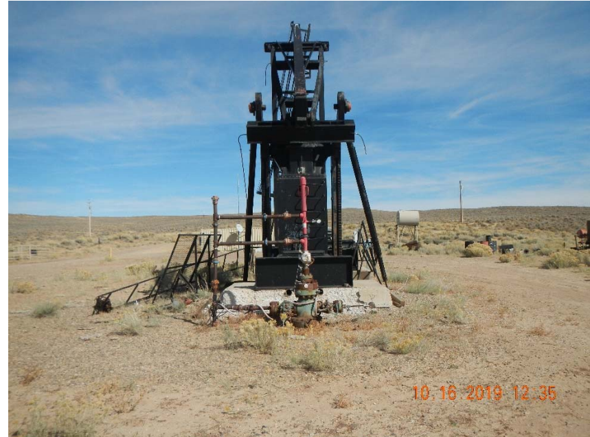
Photo 10. No wellhead sign, pump jack stored on location.
