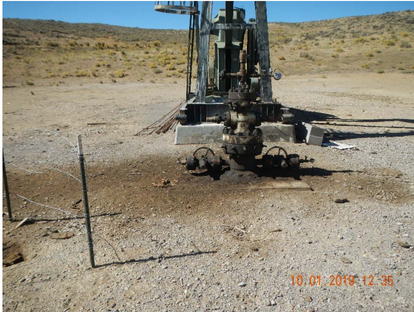
Photo 5. Stained soil at wellhead.
