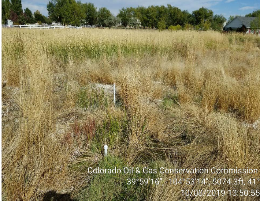
Photo 7: Temporary piezometers outside of the perimeter fence in wetland adjacent to north side of disturbed area.
