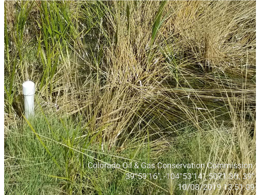
Photo 8: Temporary piezometer outside of the perimeter fence in wetland adjacent to north side of disturbed area.
