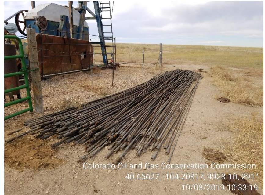
Photo 4 – Sucker Rods on the North side of the Pumping Unit
