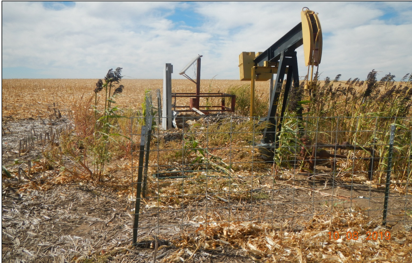
Photo 5. There debris and vegetation around the equipment which is a fire hazard. No well sign is posted.
