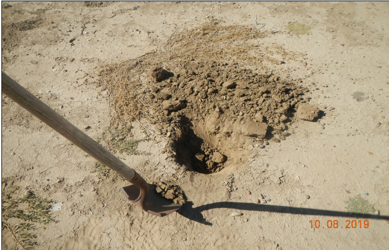
Photo 6. The top six inches did not seem to be compacted but it was much more compacted past 6 inch depth.
