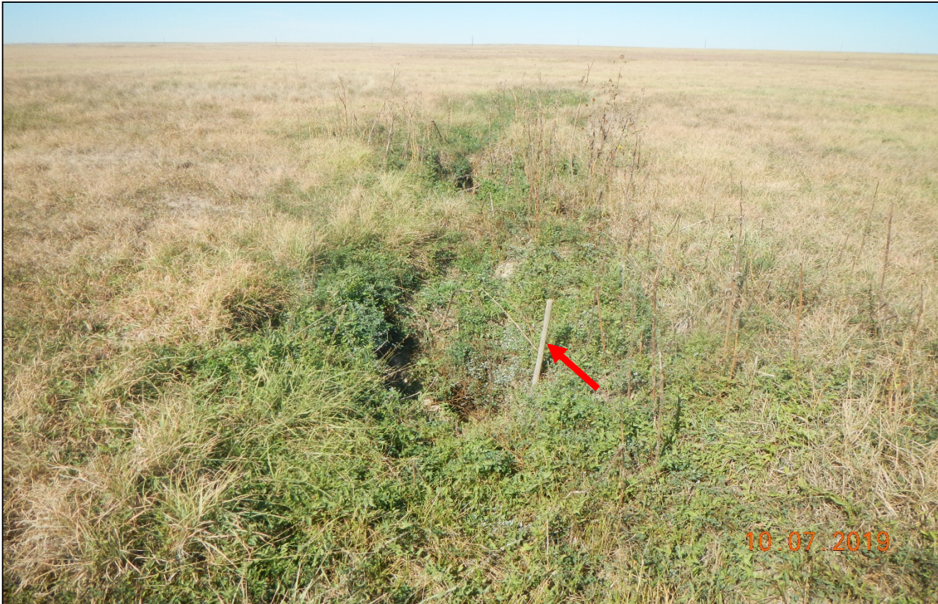
Photo 10. There is another area of subsidence at the north side of the location which is approximately 3-4ft. deep. Red arrow points to 5 ft. shovel placed in the area.
