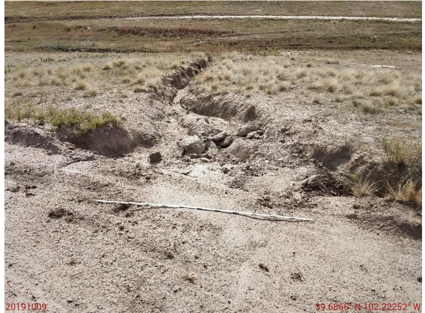
Photo 6: Photo from the south end of the location, facing south. Photo shows Operator has failed to repair/reclaim adjacent lands degraded due to stormwater runoff from the location. 6 foot measuring stick for reference.
