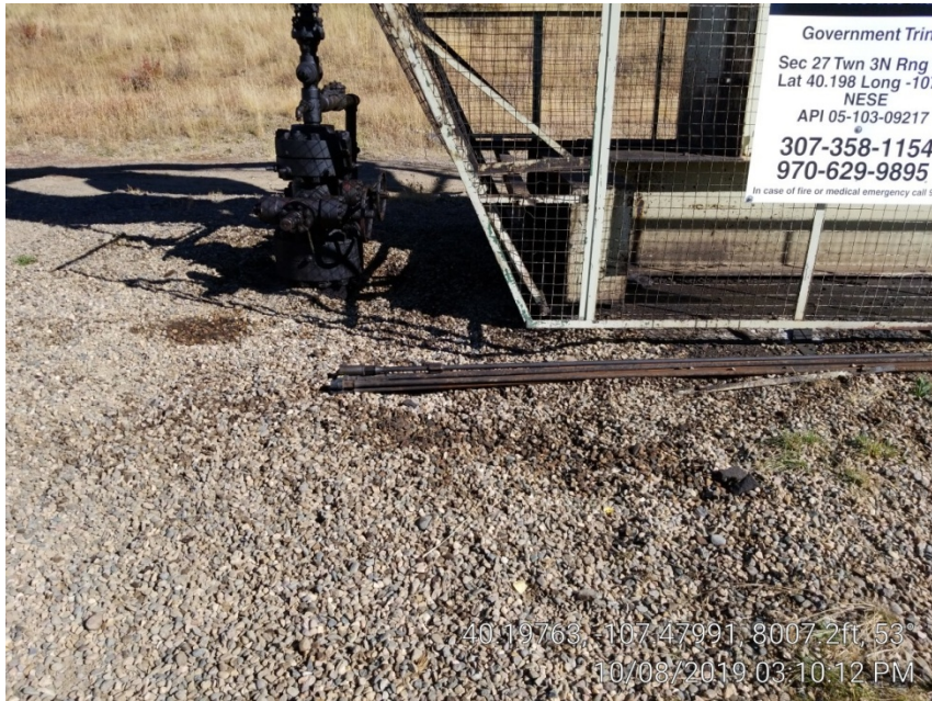
Photo 4. Stained soil at well head.
