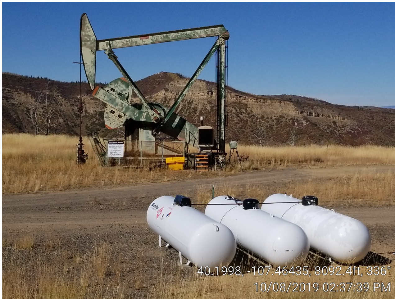
Photo 1. Pump jack & propane tanks.
