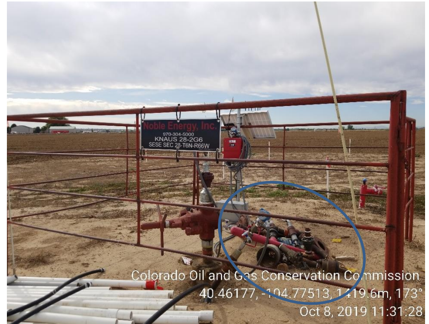
Photo 2: Wellhead; UNUSED EQUIPMENT
