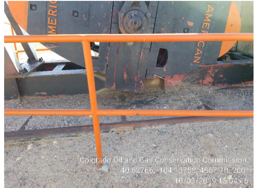
Photo 4 – Stained Soil on north side of Pumping Unit
