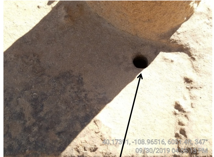
Photo 5. Casing open to atmosphere.
