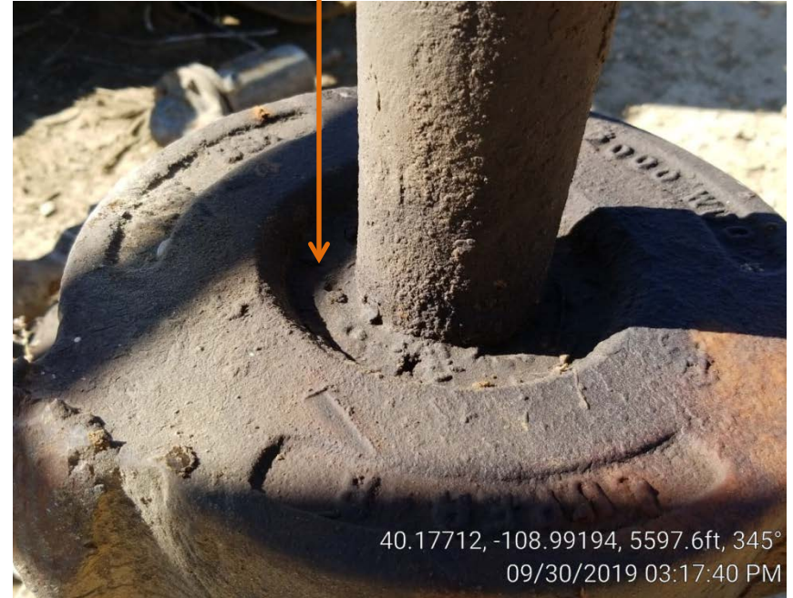
Photo 5. Well head gas leak.
