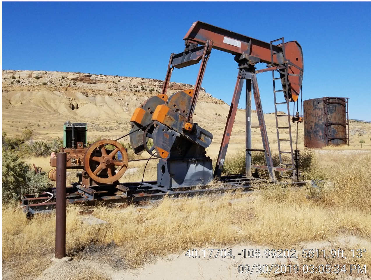
Photo 2. Pump jack & portable tank.
