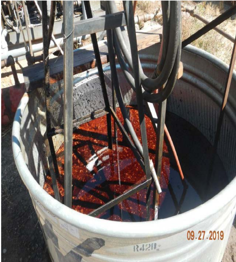
Photo#11: Stock tank used for containment of day tanks.
