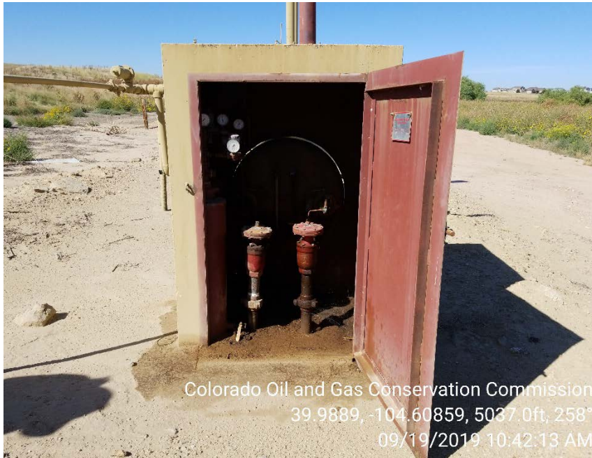
Photo 5 – Stained soil at separator
