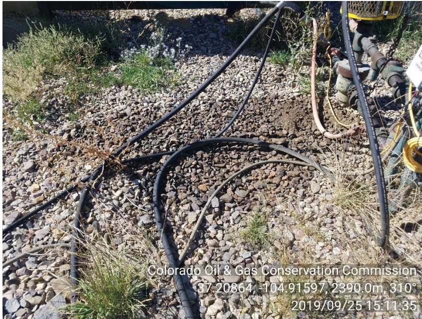
PHOTO 3: AREA OF STAINED SOIL APEARS TO BE FROM HYDRAULIC HOSES OR DRIVEHEAD FITTING. "Properly treat or dispose of oily waste in accordance with 907.e." CA DATE 10-25-19
