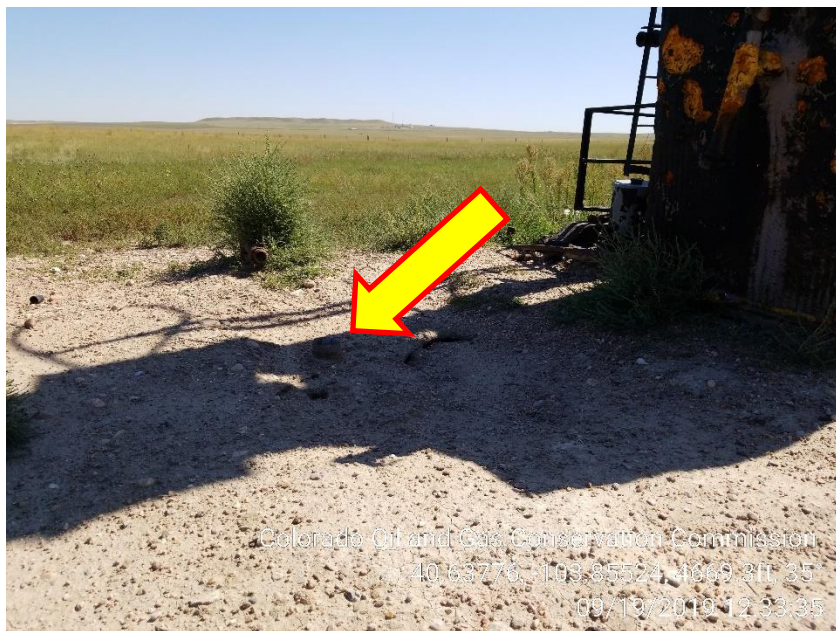
Photo 5 – Open well bore, needs Nightcap or Cut and Capped
