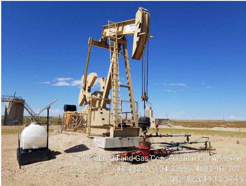
Photo 1 – Pumping Unit, weeds around well
