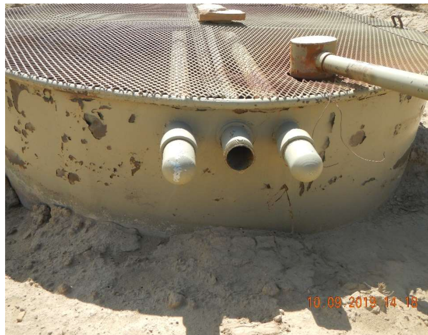
Photo #10 – View of the uncapped flowline on the 60 bbl produced water tank.
