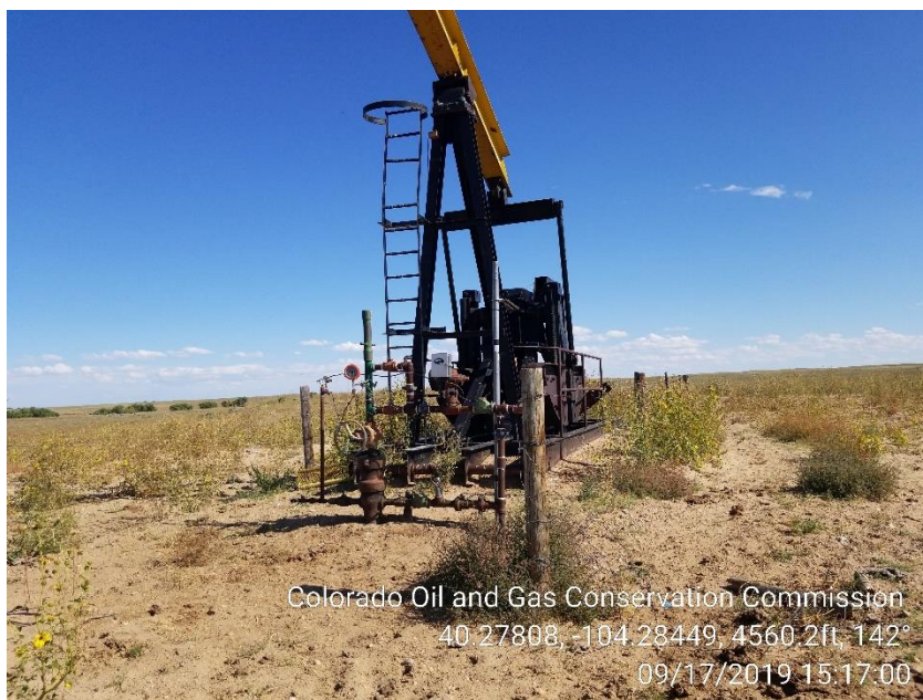
Photo 1 – Wellhead and Pumping Unit, weeds around well
