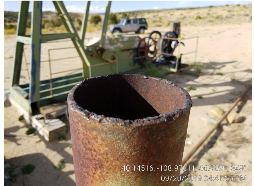
Photo 6. Stack by pump jack without bird screen.
