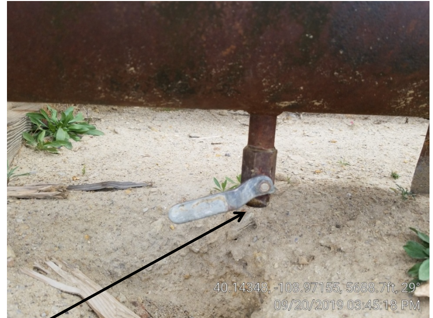
Photo 4. Pump jack casing gas tank valve.
