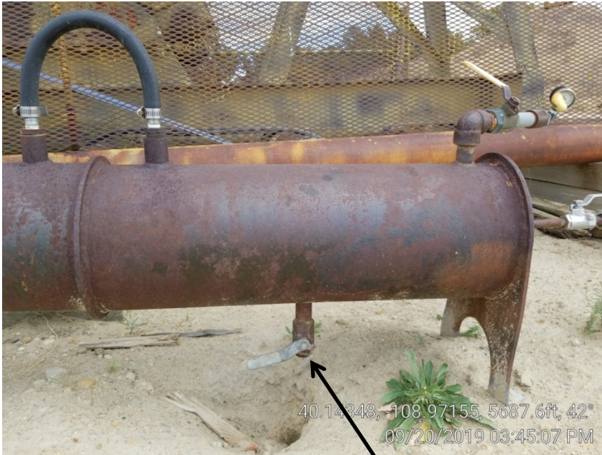
Photo 3. Pump jack casing gas tank.
