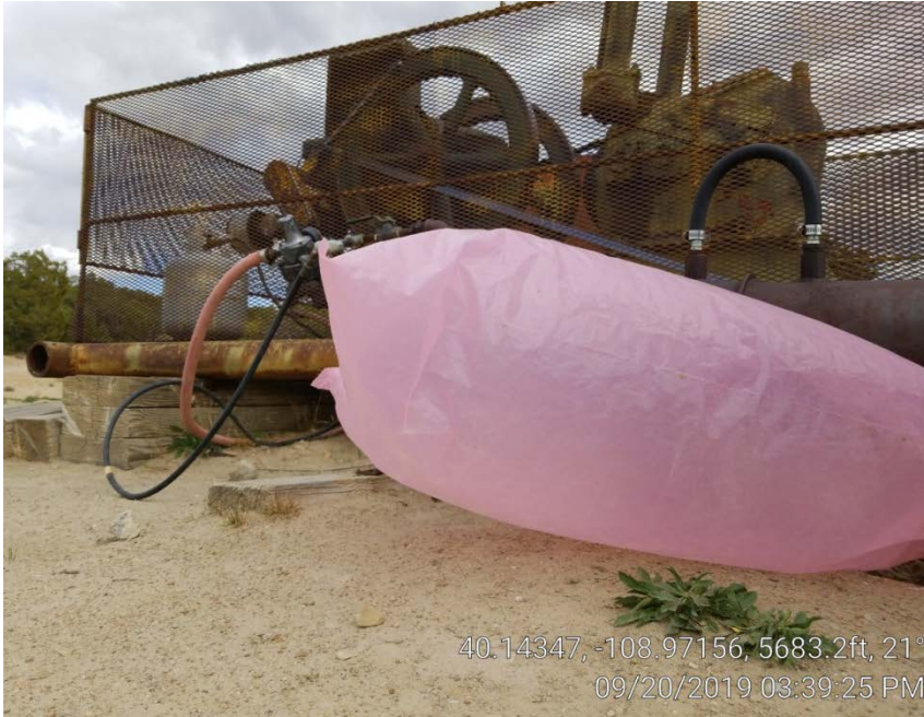
Photo 5. Bag on pump jack casing gas tank valve.
