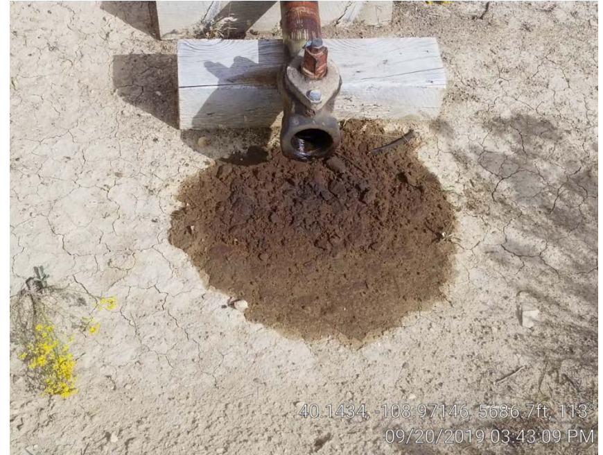
Photo 6. Stained soil at crude off loading valve.
