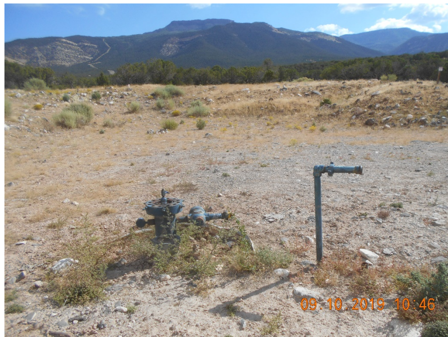
Location overview from SW side of wellhead looking NE. Unused 2" riser. Open ended.
