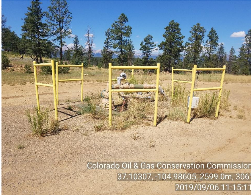
PHOTO 1: WELLHEAD/ WEEDS AROUND WELLHEAD. CUT WEEDS AND MAINTAIN WEEDS AROUND EQUIPMENT IN ACCORDANCE WITH RULE 603.f. CA DATE 10-6-19
