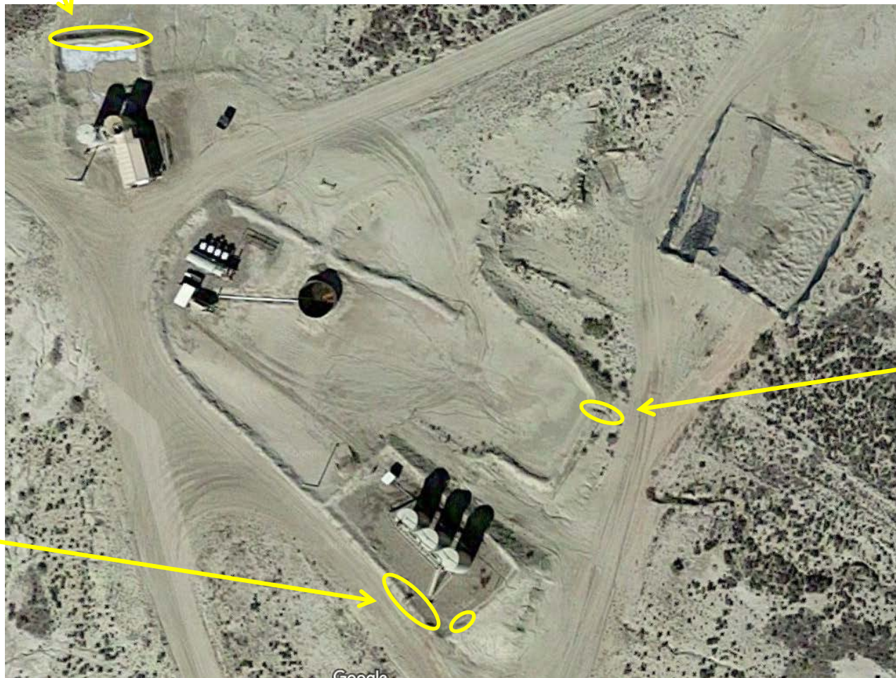
Photo 8. Tank battery – Inadequate berms circled in yellow.
