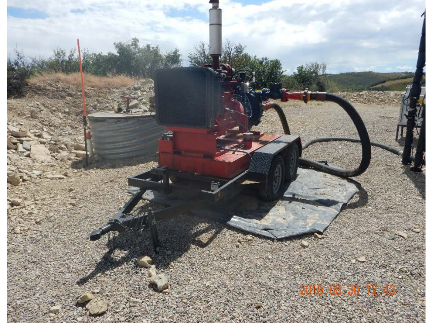
Photo #8 – Pump trailer with lined containment located east of tank battery.
