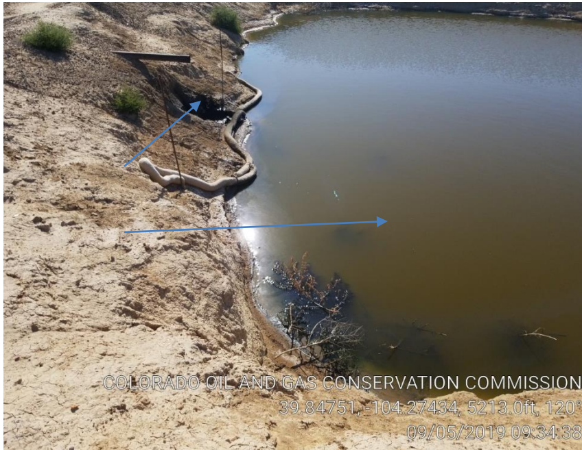
Pic 15 hydrocarbons in pit/stained soil
