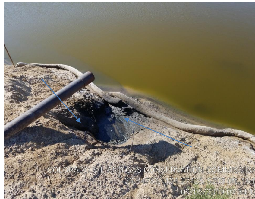
Pic 14 hydrocarbons in pit / stained soil
