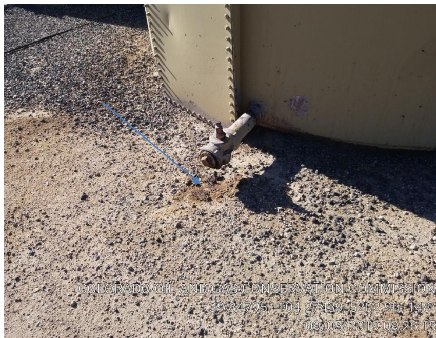
Pic 3 stained soil/mechanical conditions
