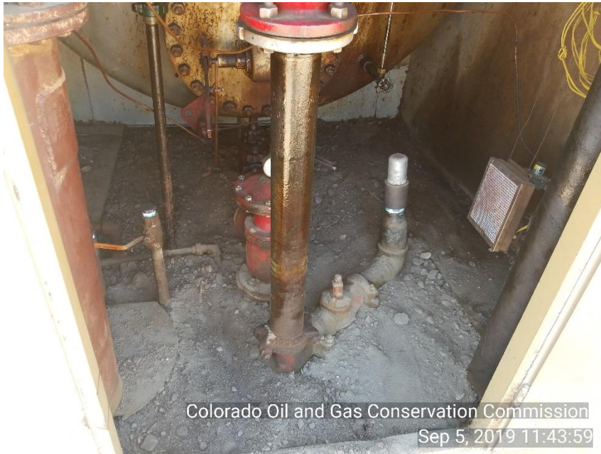
Photo 3 Stained soil appears to have been removed from separator
