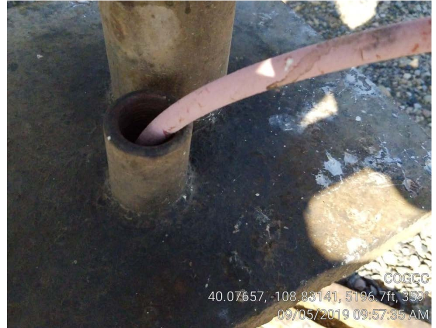
Photo 3. Casing open to atmosphere.
