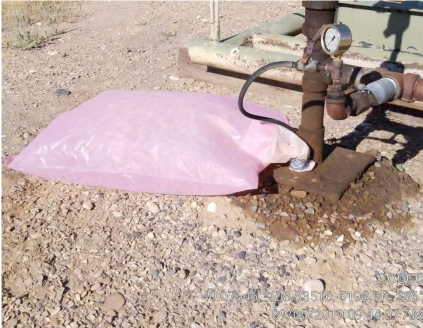
Photo 4. Bag attached to venting gas.
