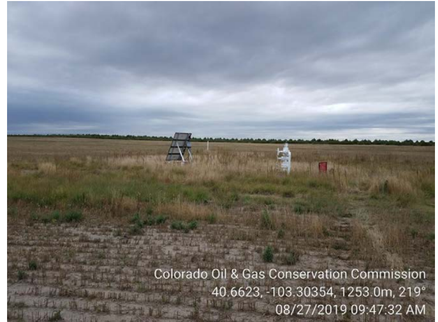
2. Wellhead, solar powered cathodic rectifier and vegetation
