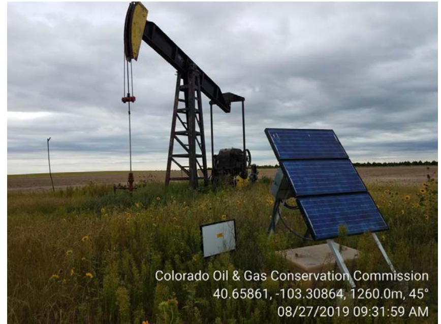
2. Unit, solar powered cathodic rectifier and vegetation
