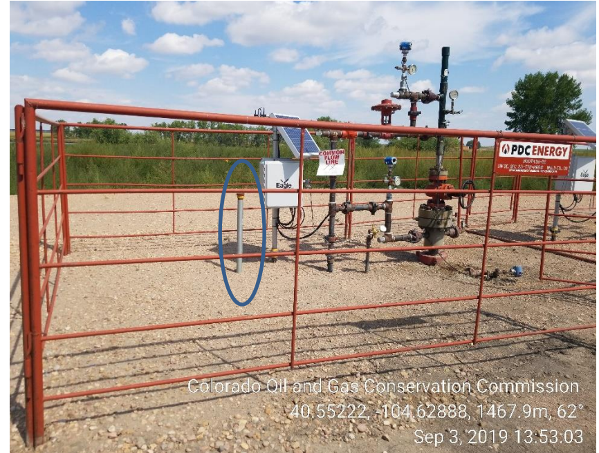
Photo 2: Wellhead; unused riser
