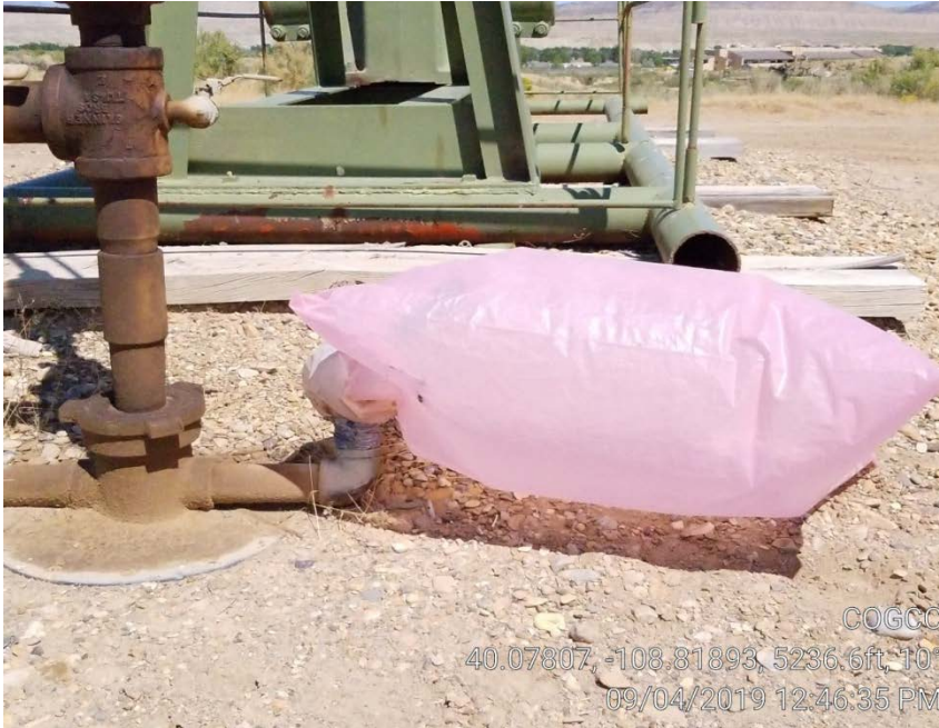
Photo 4. Bag attached to venting gas.
