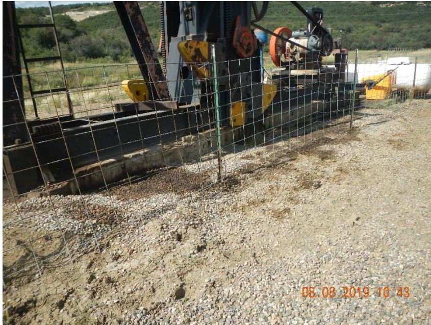
Photo 3. Stained soil at pump jack motor.
