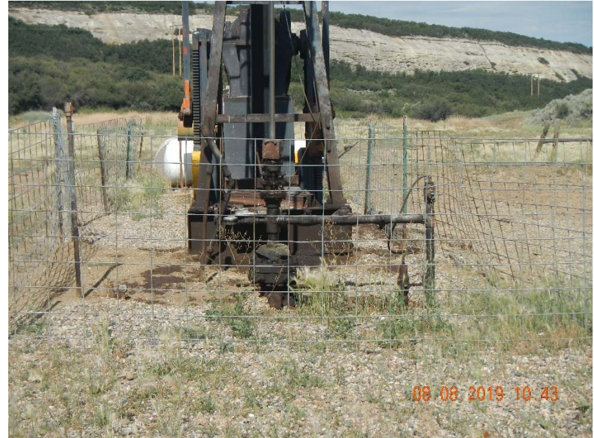
Photo 2. Stained soil with fresh soil on top of it at wellhead.
