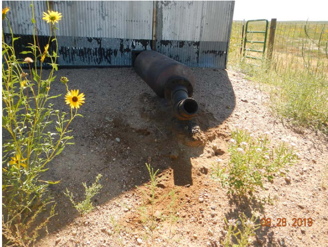
Photo # 2 - 05-121-07069 - Oil stained soil at exhaust
