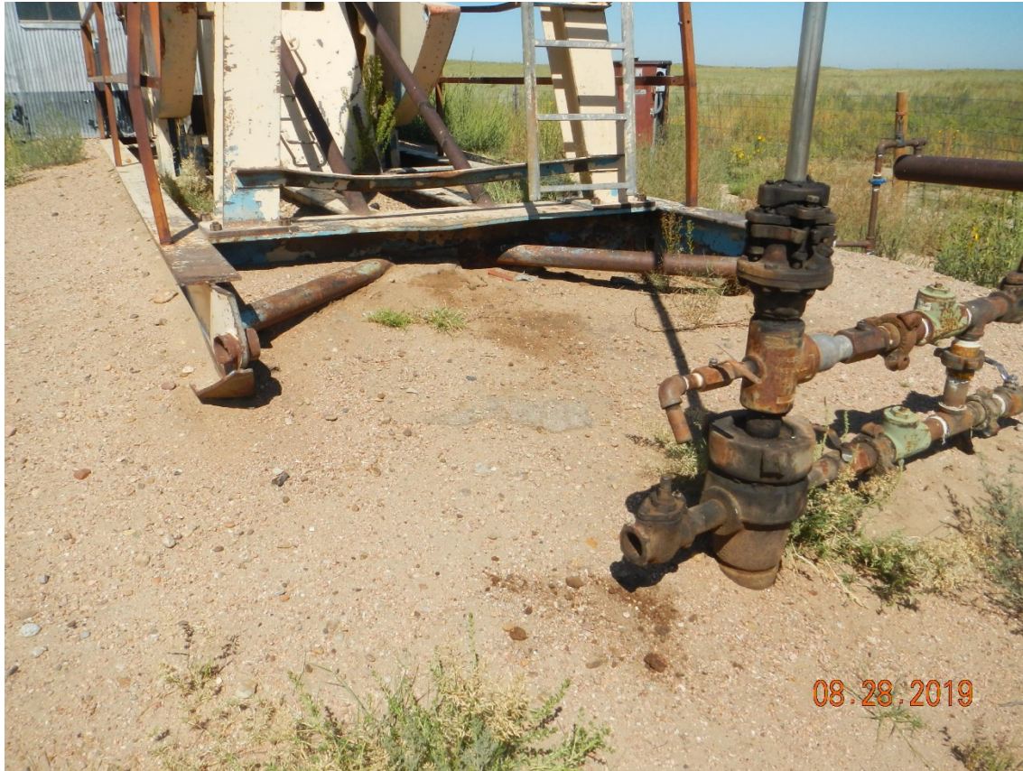
Photo # 4 - 05-121-07069 - Oil impacted soil near wellhead
