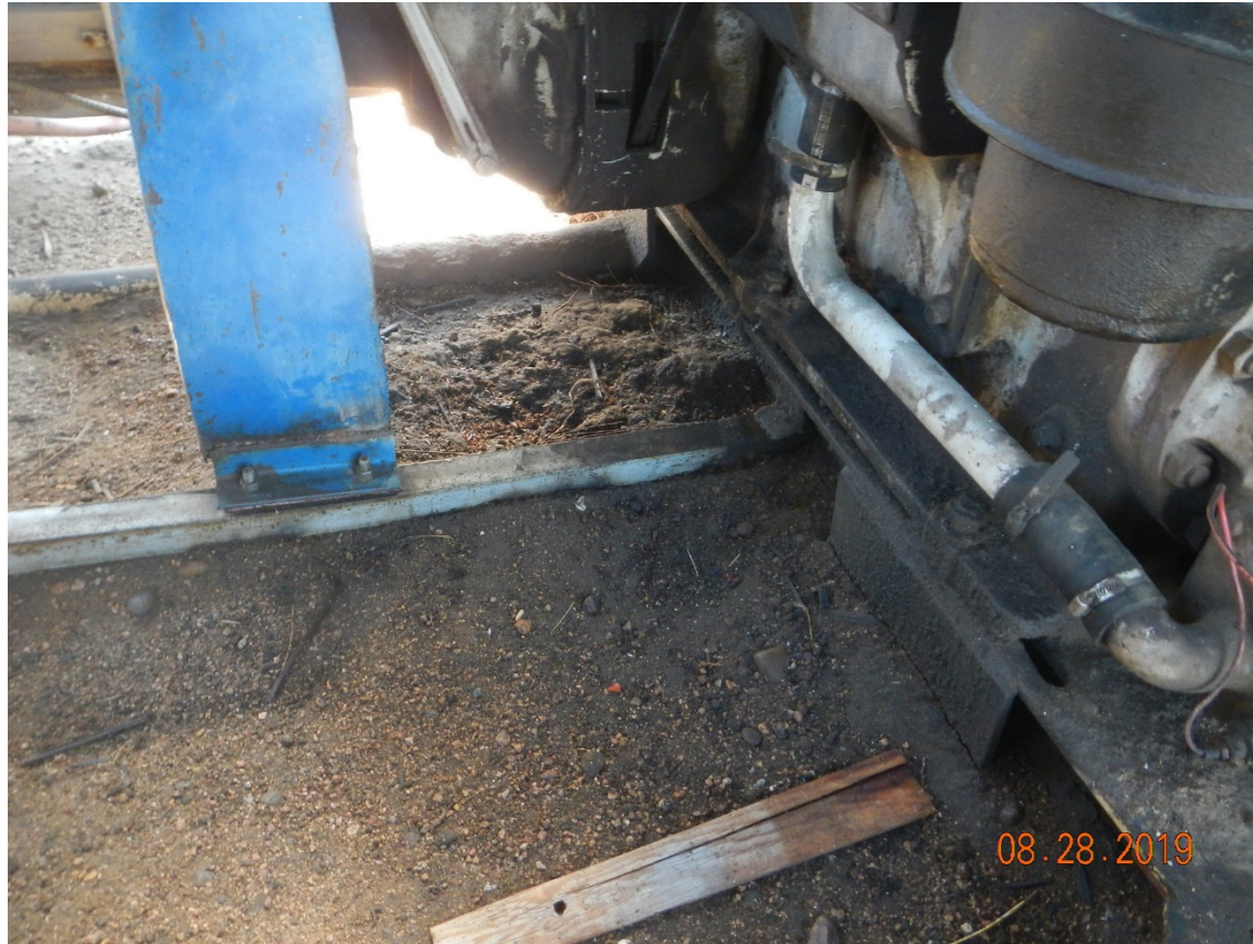
Photo # 4 - 05-121-07069 - Oil impacted soil near motor
