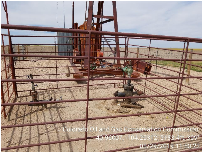
Photo 1 – Pumping Unit, Well is TA'd
