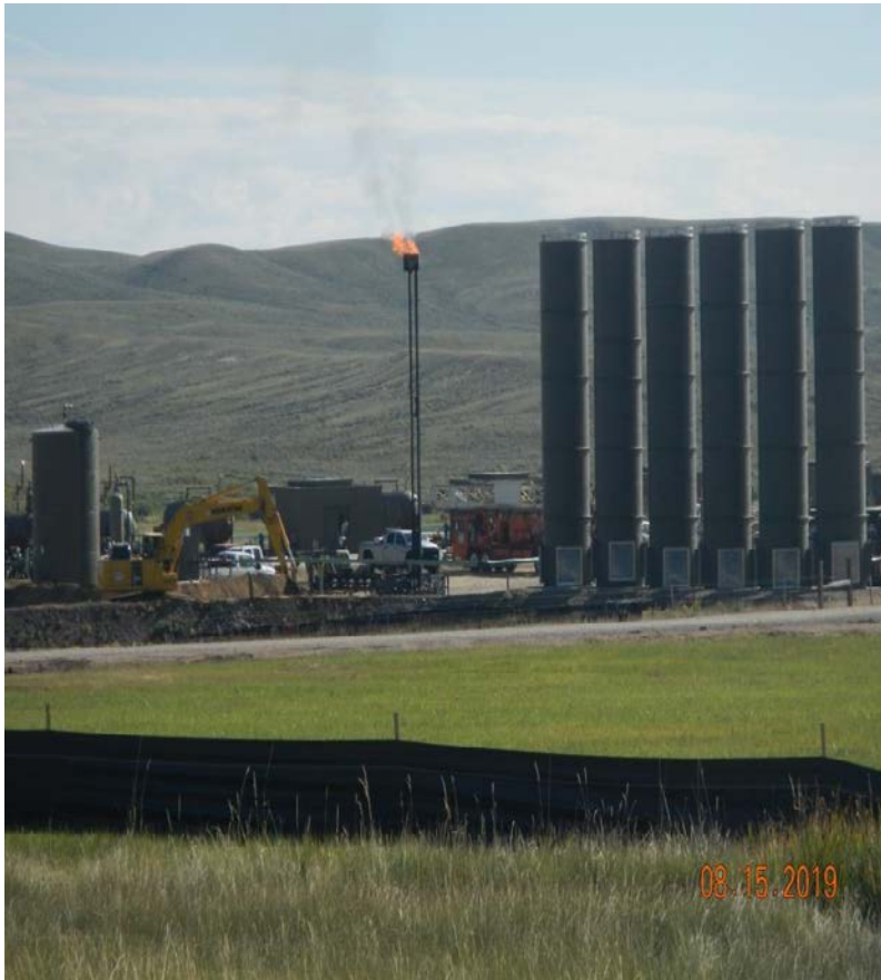
Photo#1: View of Location to Northeast. Flare did not seem to be burning efficiently.
