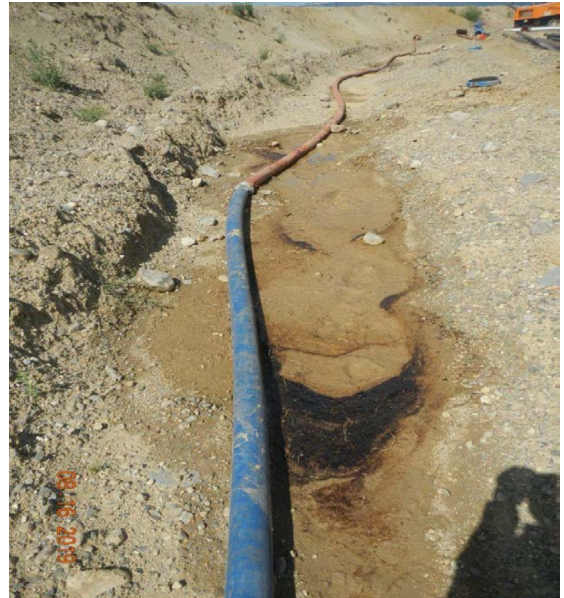
Photo#8: Stained soil at South edge of pad along lines laying on ground, running East-West.
