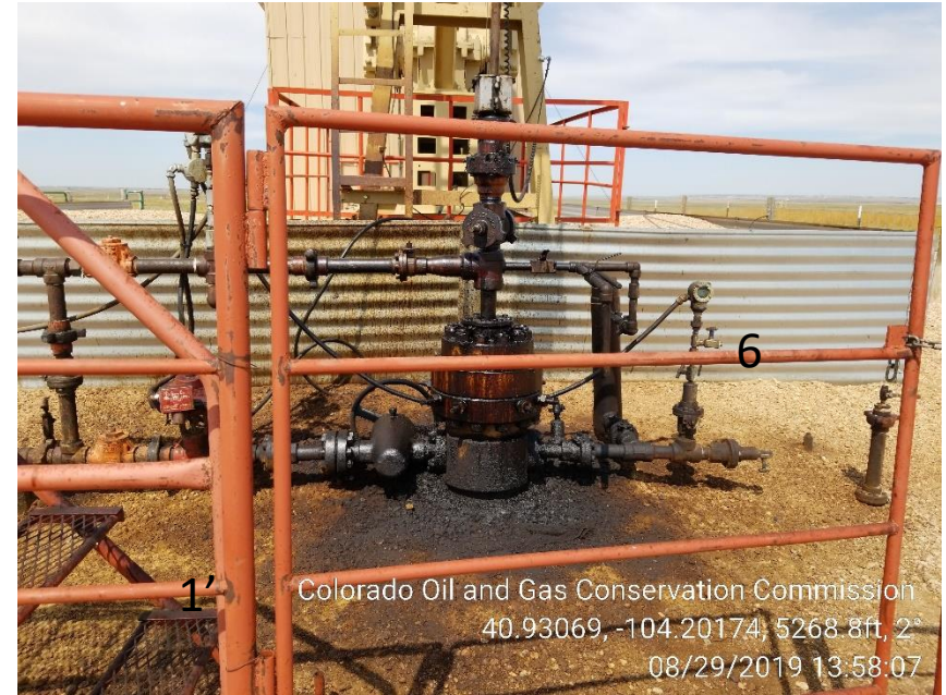
Photo 2 – Stained Soil at Wellhead approximately 12' x 6'
